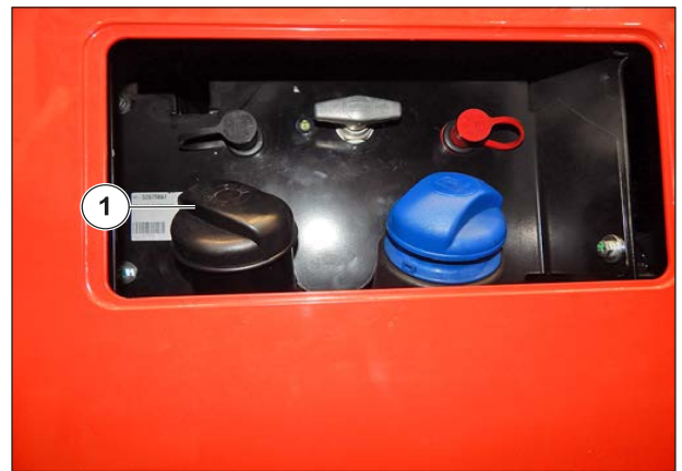
Figure 121: Filling the fuel tank
