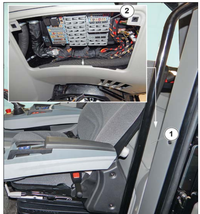
Figure 214: Fuse and relay in cab
