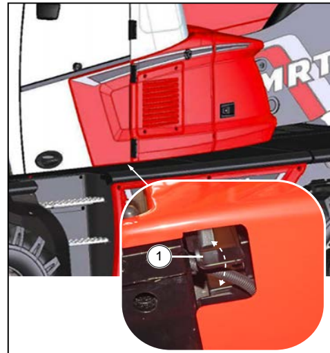
Figure 61: Door window release lever from outside cabin
