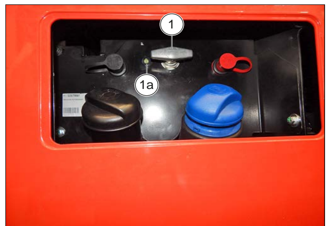
Figure 66: Battery disconnect switch
